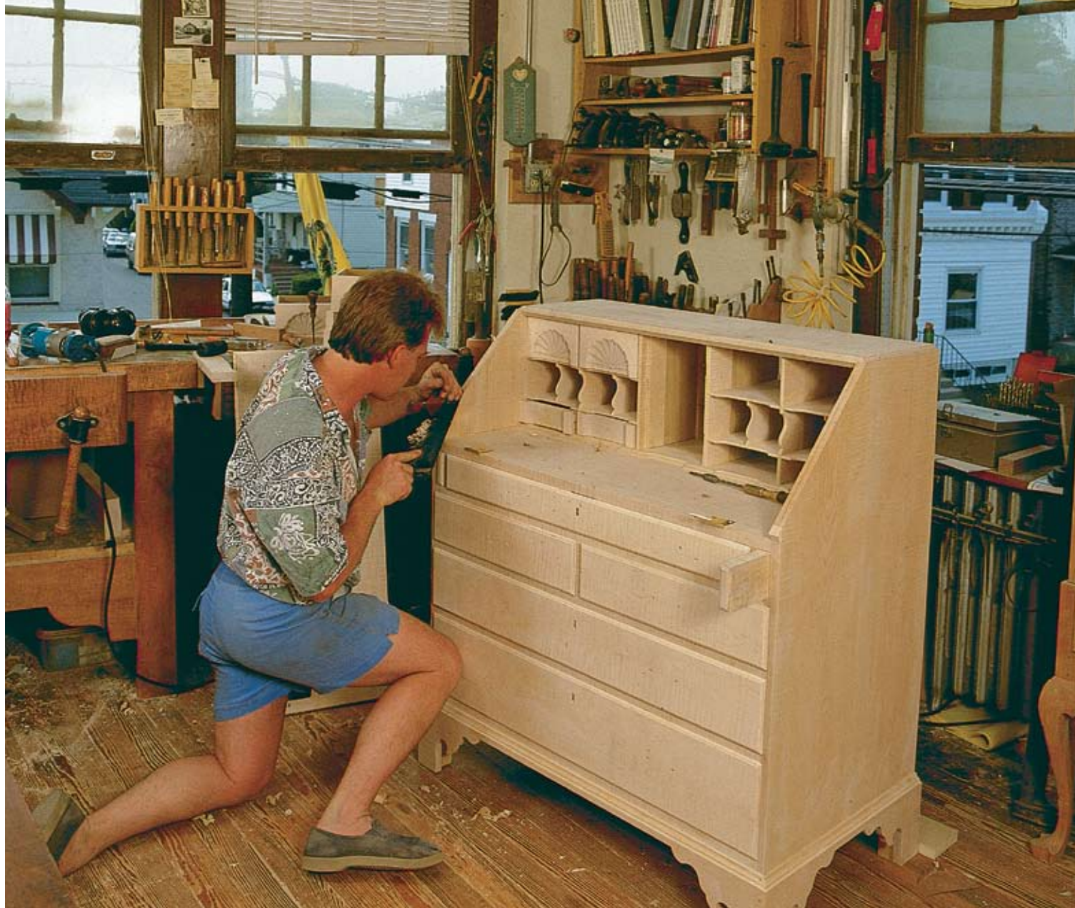
Reproducing furniture with a reproduction plane —Gerald Martin, building an 18th-century Chester County slant-top desk, smooths end grain with a reproduction Stanley #9 plane made by Maine planemaker Lie-Nielsen.
